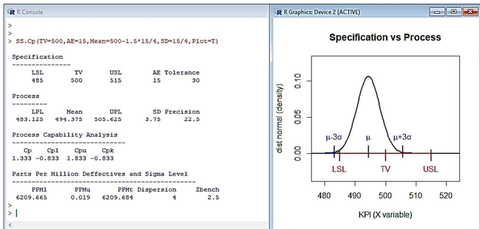
Figure 2 – Output of Function *SS.Cp*, Showing a Process with a  $1.5\sigma$  Shift to the Left of the TV, with  $\sigma = AE/4$ . The Dispersion is 4,  $C_p = 1.33$ ,  $C_{pK} = -0.833$  and 6200 PPM are Produced, leading to a  $Z_{bench} = 2.5$
