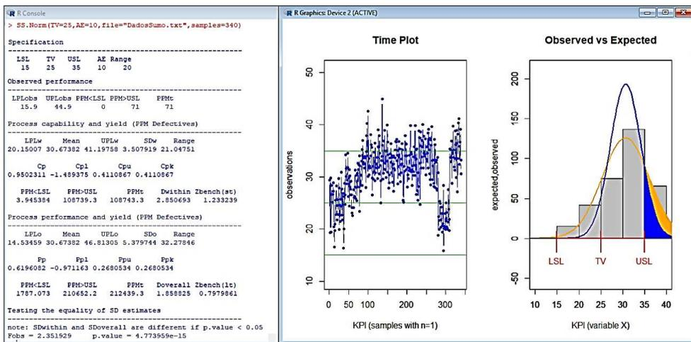
Figure 3 – Output of Function SS.Norm, Showing a Real Industrial process dealing with Daily Losses in Juice Production. The Process has Very Low Performance ( $Pp = 0.62$ ) and is Displaced towards the Right ( $Pp_K = 0.268$ ), Producing 108743 PPM Corresponding to a Long Term Sigma Level of 0.798. There are Evident Special Causes of Variation ( $p = 4.773959 \times 10^{-15}$ ), and a  $Cp = 0.95$  Shows a Need for Improvement
