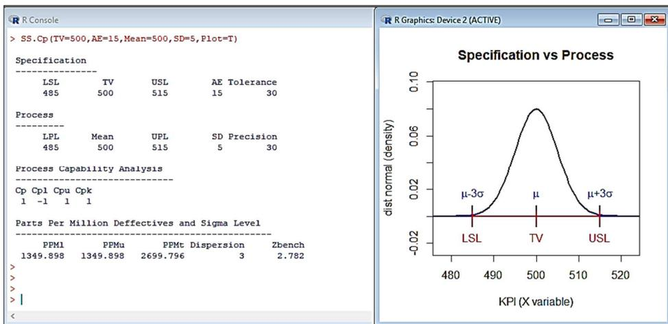
Figure 1 – Output of Function *SS.Cp*, Comparing a Process with  $\mu$  Adjusted to *TV*, and with  $\sigma = AE/3$ . The Dispersion is 3,  $Cp = CpK = 1$  and 2700 PPM are Produced, Corresponding to a  $Z_{bench} = 2.78$ . The Process Parameters  $\mu$  and  $\sigma$  are not Calculated, but Stipulated by the User
