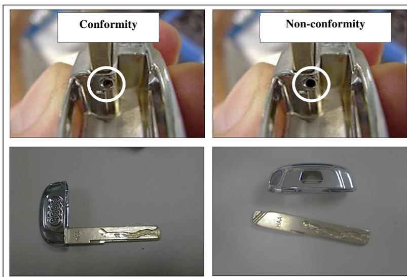
*Figure 1 – Visualization of Missing Pin*
