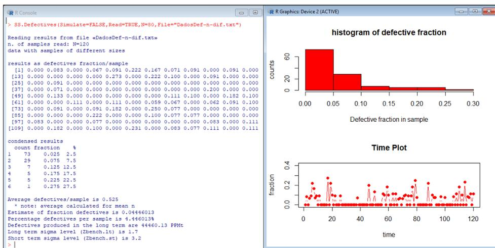
Figure 5 – Output of Function *SS.Defectives*, Showing a Real Industrial Process, Analysing Samples of Different Sizes of Pre-Packaged Coffee Beans. Units with Contents Lower than the Legal AE or Higher than the Internal AE, Are Defective.  $Z_{bench(LT)}$  Shows Possibilities for Improvement
