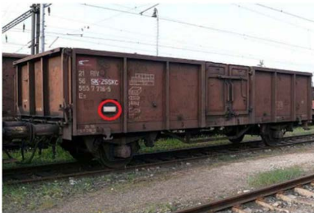
Figure 2 Possible placement of RFID tag in real conditions [3]
