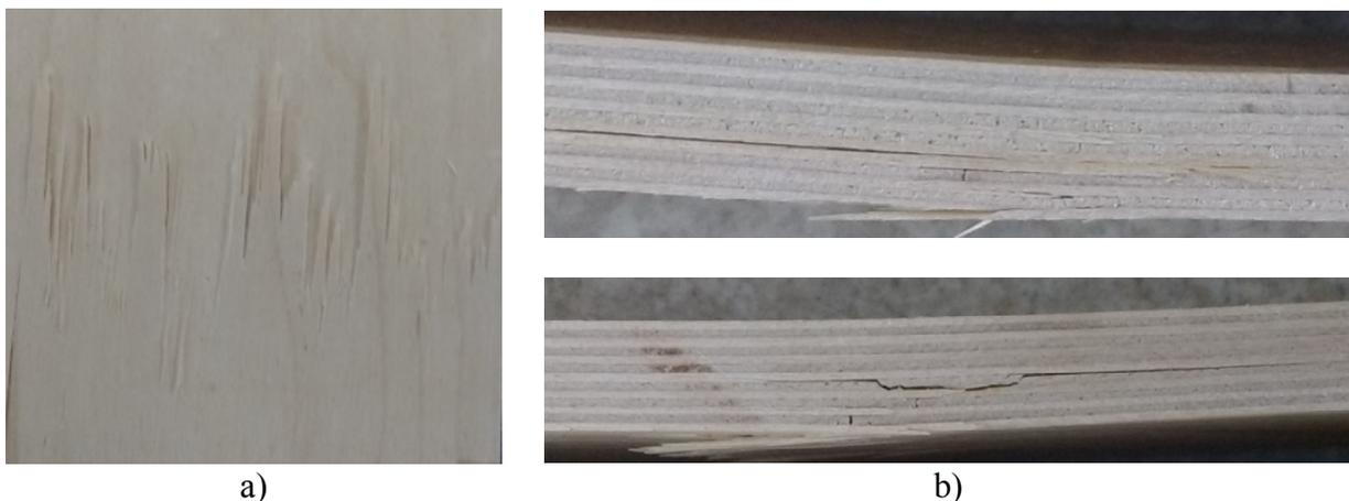
Fig. 4: Failure mode for wood particle board specimens: a) top view, b) side view.
