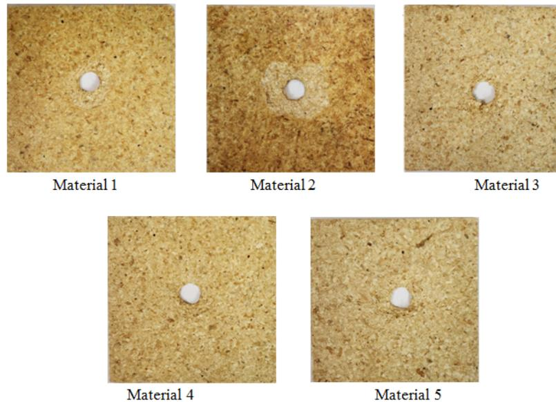
*Fig. 5: Damage views of the impacted bio-composites.*
