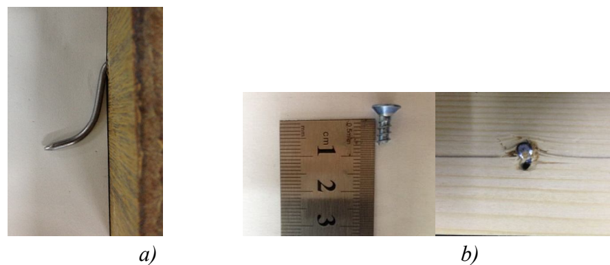
Fig. 5: Failure modes of the joints with PSB sheathing: (a) bending of fastener, (b) brittle failure of screw.
