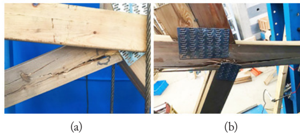
Fig. 6: Wood tearing failure under loading B-joint: (a) front, (b) back.
