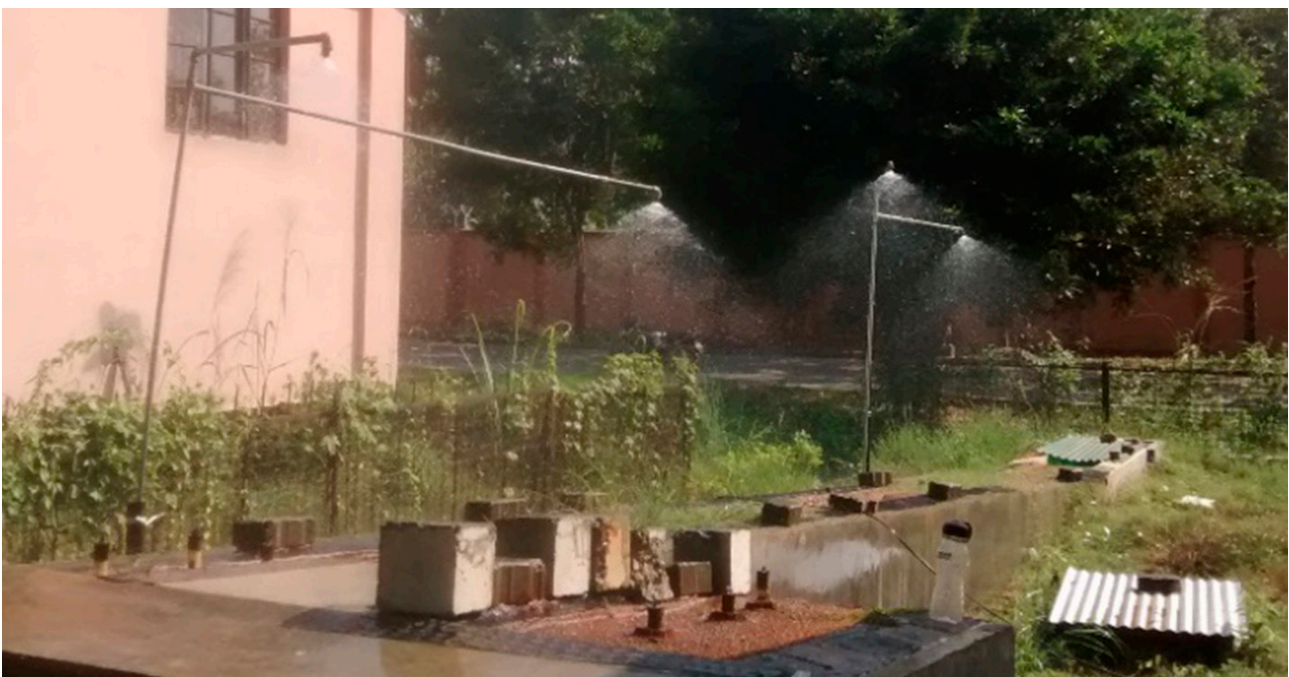
Figure 1 MLCS test setup during a rainfall simulation event
