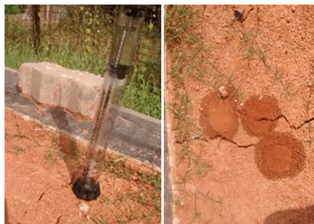
Figure 4 Repeated infiltration measurements around desiccation cracks on surface soil
