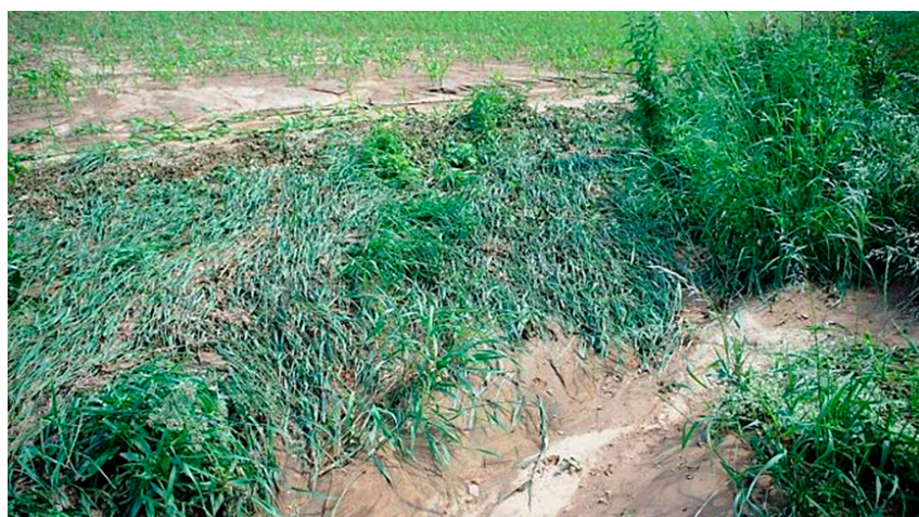
Figure 4 Exceeding of sediment trap capacity of local grass filter strip after rainfall event Photo: Aydin, 2017
