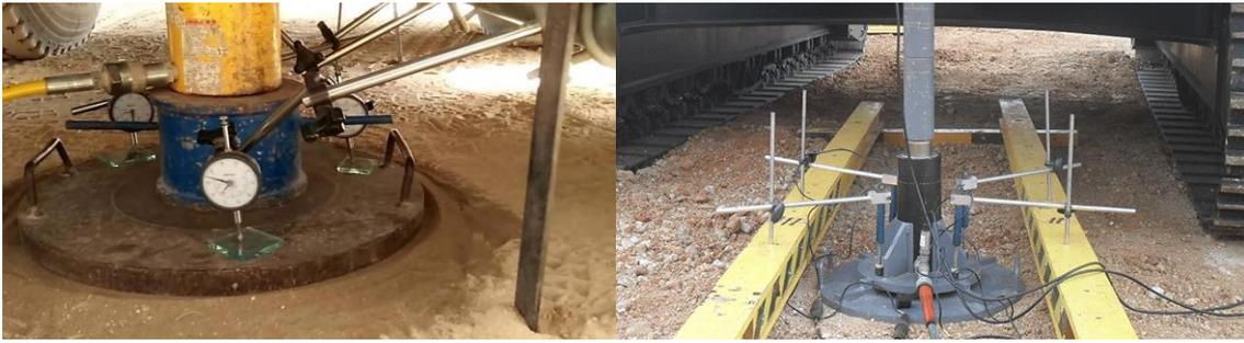
Figure 4: Plate load tests on stone columns
