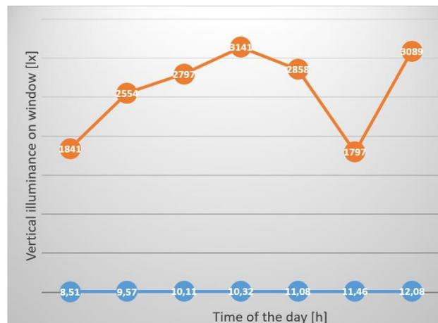
Figure 5: Vertical photopic illuminance of the window during measurements on November 3, 2021
