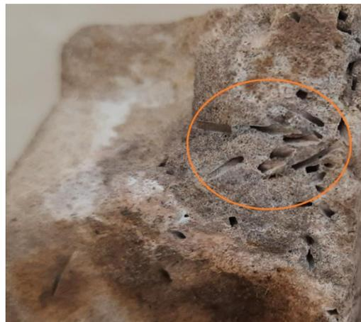
Figure 11: Formation of voids in the M5 mortar matrix after heating at 400 °C
