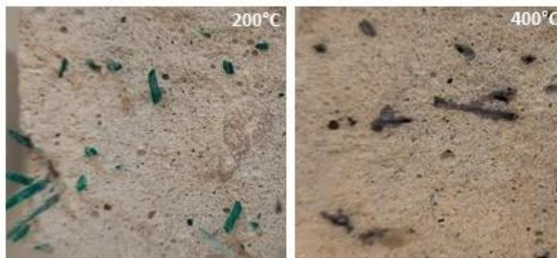
Figure 5: The visual state of the mortar M<sub>2</sub> at a temperature of 200°C and 400°C
