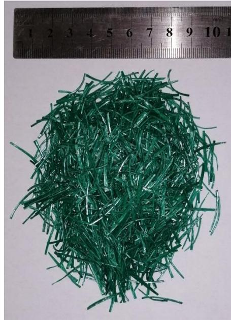
Figure 3: PET strap waste fibers used
