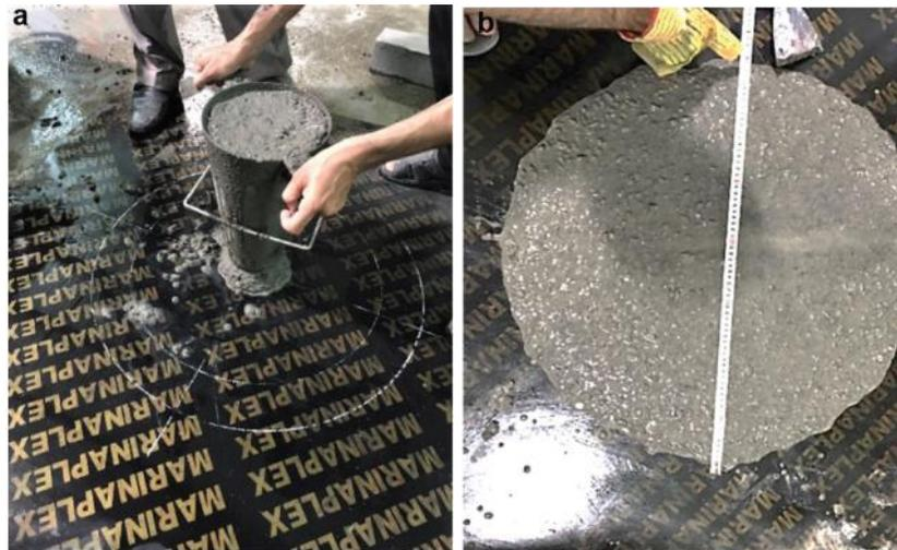
Figure 1: a) Slump flow test, b) Slump diameter measurement
