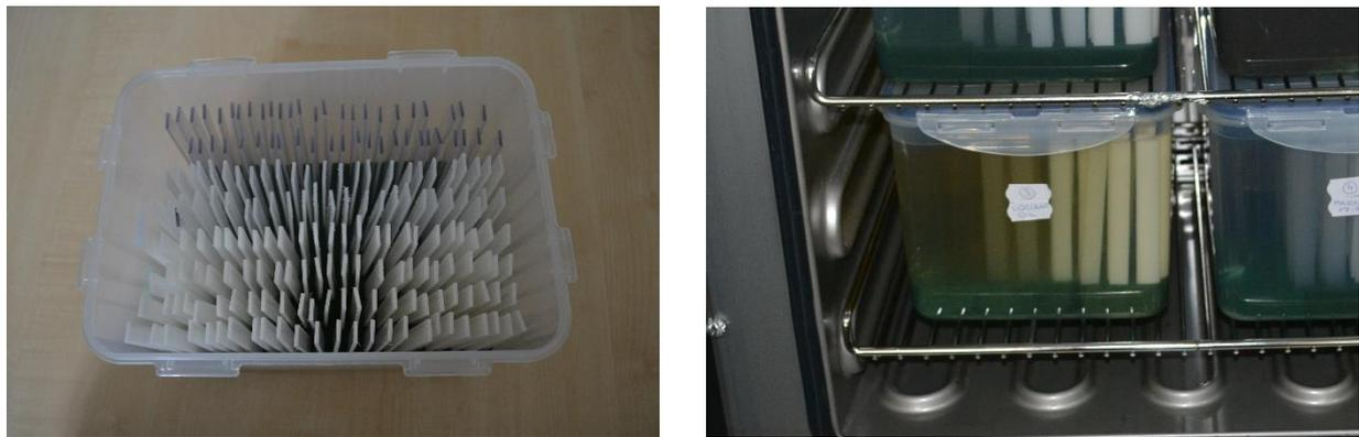
Figure 3: Plastic samples in the test beakers: (a) Samples before immersion in coconut oil and thermal cycling; (b) Samples immersed in coconut oil placed in a small environmental chamber
