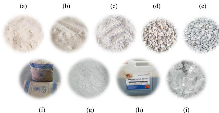
Figure 1: The materials used for making the various concretes studied. (a) Dune sand, (b) Natural sand, (c) Quarry sand, (d) Gravel 15/25, (e) Gravel 5/15, (f) Cement CPJ-CEM II/ A 42.5, (g) MEDAPLAST H silica fume, (h) MEDAPLAST-SP 40 super-plasticizer, (i) SIKAFIBRE Polypropylene 12/32
