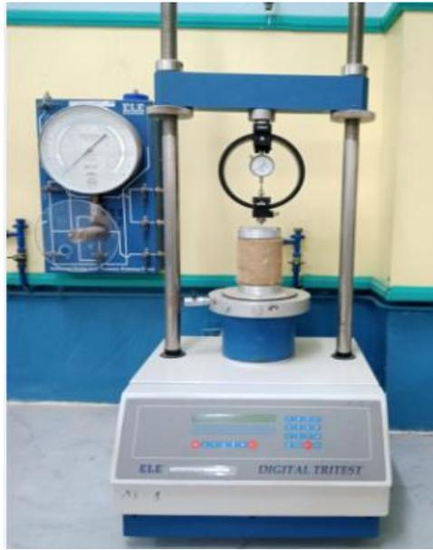
Figure 3: Simple compression device
