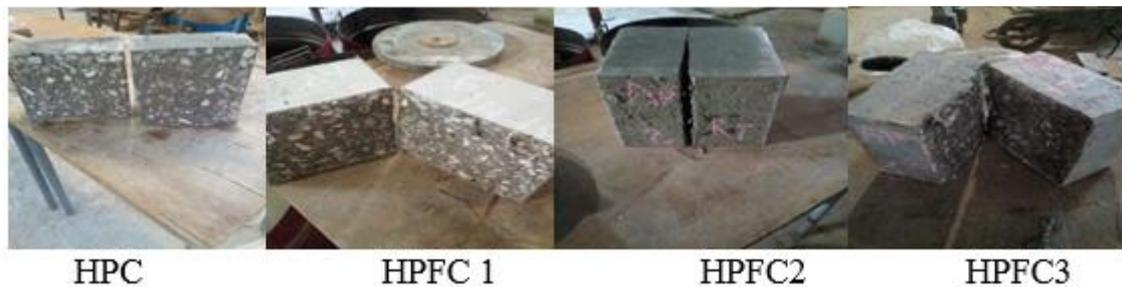
Figure 8: Failure of tensile test pieces by splitting different concrete at 20°C
