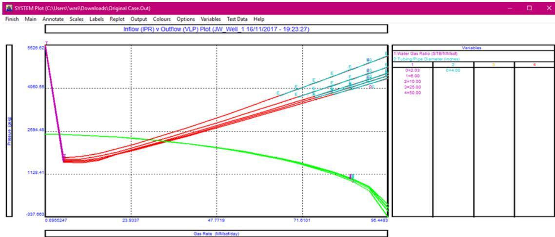
Fig. 6. System plot showing impact of WGR on liquid loading
