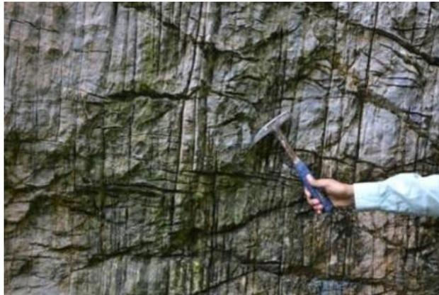
Figure 2 Intensely fractured tight Carboniferous limestone in NW Malaysia. Similar fractured basement rocks produce hydrocarbons in SE Asia.
