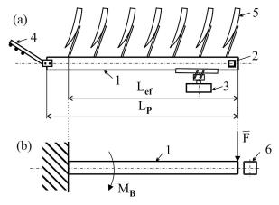
Figure 4 Plough and its model (a) 1-plough beam, 2-acceleration gauge, 3-wheel, 4-three point linkage mechanism, 5-body (b) 1-plough beam, 6-beam profile,  $\overline{F}$ -force,  $\overline{M}_B$ - bending moment
