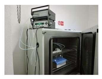
Figure 1 Sample of litter placed in a climatic chamber and instrument for measuring gas concentrations
