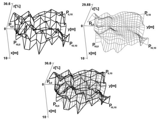
Fig. 3 Control points, B-spline surface of order (2, 2) and their comparison.
