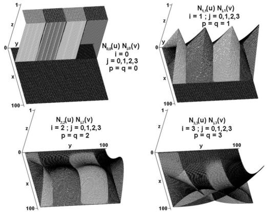
Fig. 1 Basis functions of the B-spline surface.
