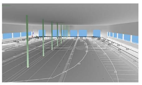
Figure 8 View into the stable with the worst daylighting - solution I. Source: authors
