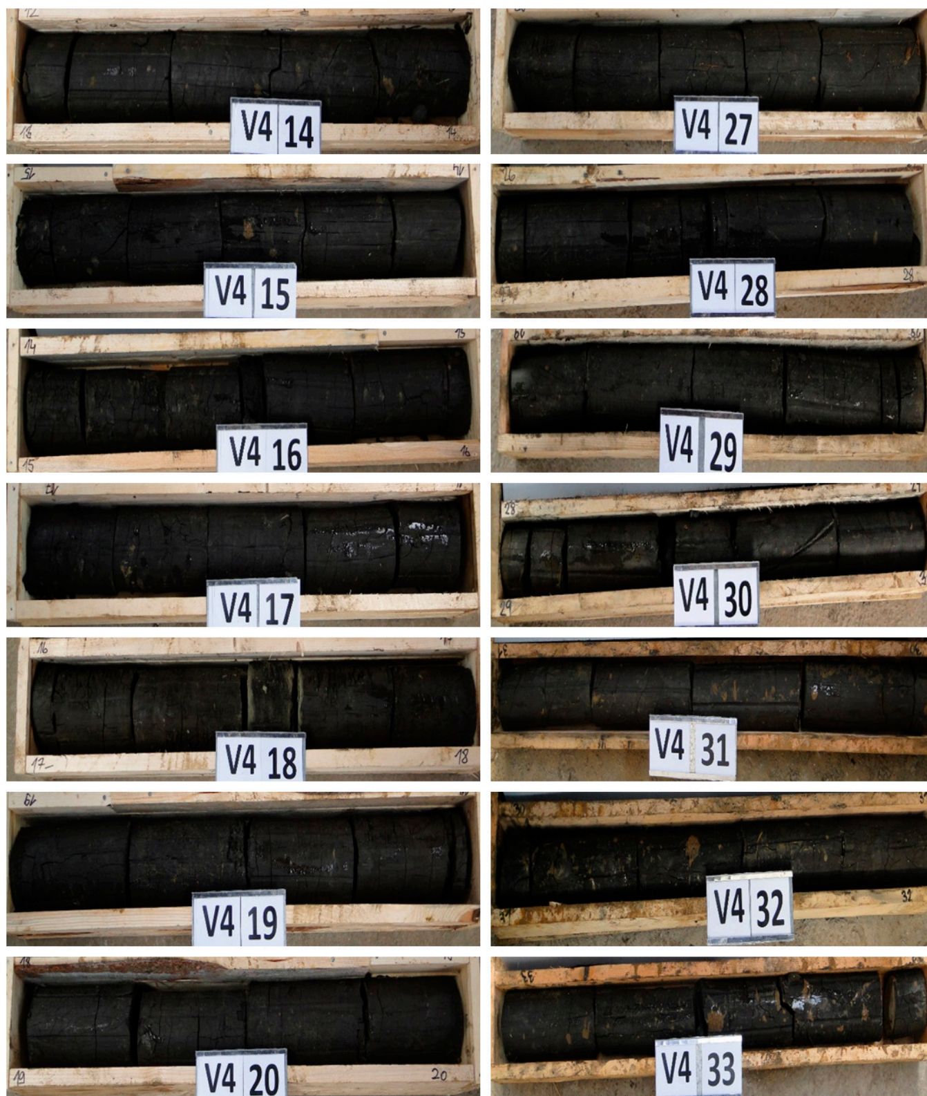
Figure 3 Colour of wet alginite samples obtained from different depths at the Pinciná deposit (Photo: A. Oravec, 2020)
