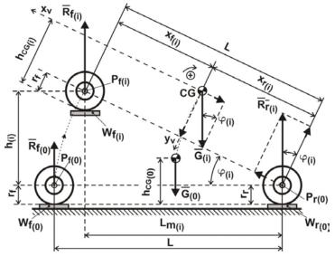
Figure 5 Machine in lifting position
