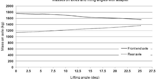
Masses on axles and lifting angles with adapter
