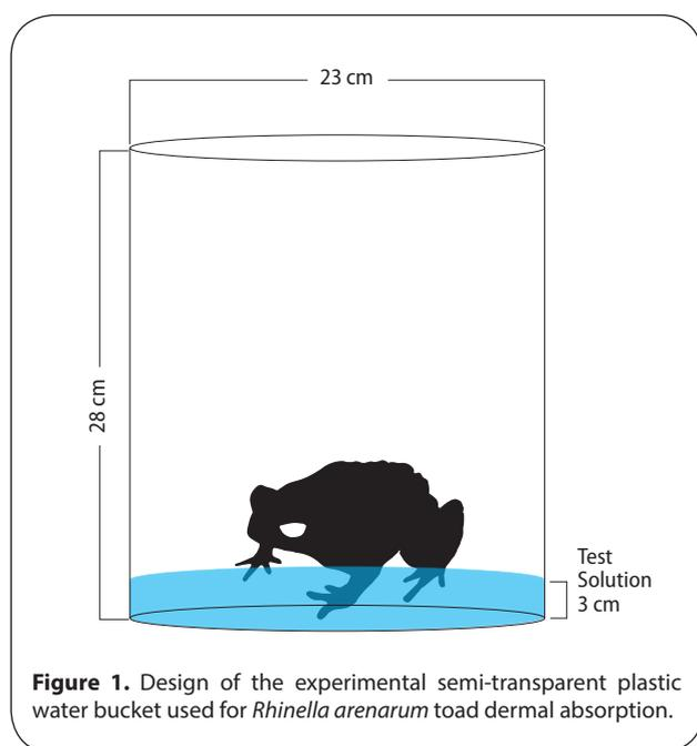
**Figure 1.** Design of the experimental semi-transparent plastic water bucket used for *Rhinella arenarum* toad dermal absorption.
