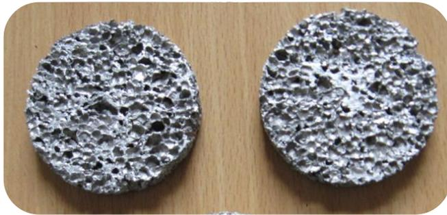
Figure 8 Aluminium foam samples
