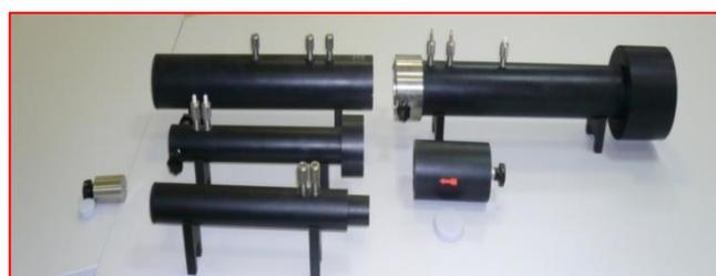
Figure 1 The impedance tube [6]
