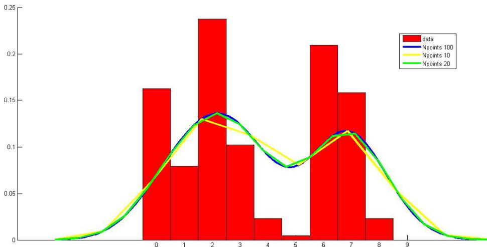
**Figure 6** Histogram of the daylight factor together with Kernel distribution estimation for different numbers of approximate points
