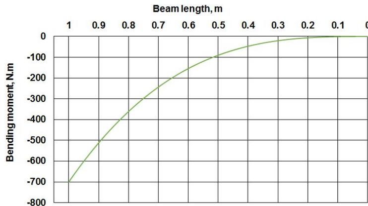
Figure 2 Bending moment function visualization
