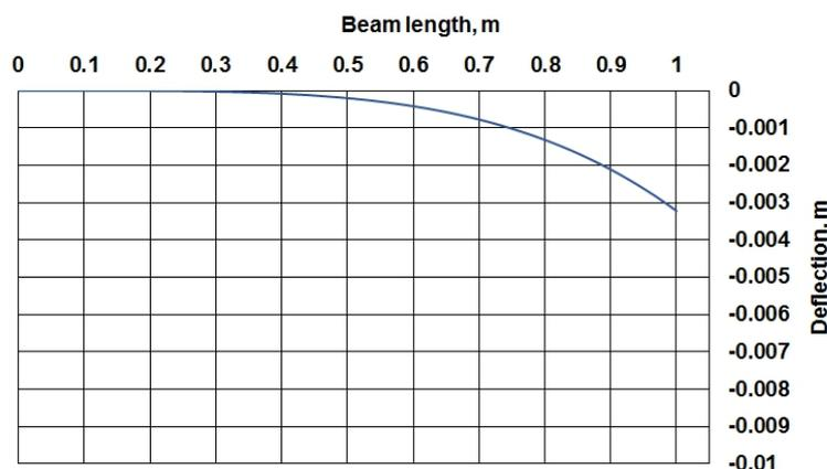
Figure 3 Deflection curve of the loaded beam from exact solution
