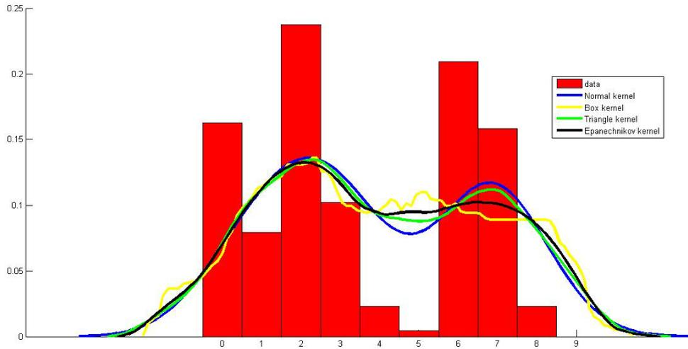
**Figure 5** Histogram of the daylight factor together with Kernel distribution estimation for different types of kernels
