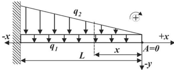
Figure 1 Model of loaded beam
