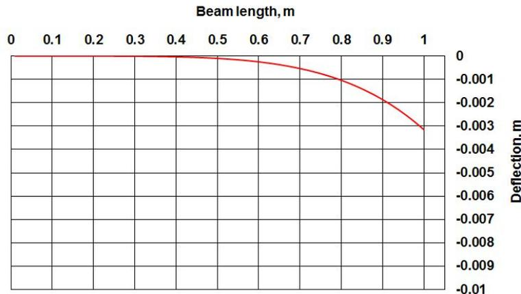
Figure 4 Deflection curve obtained by numerical integration
