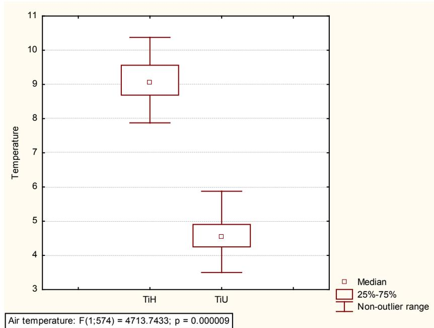
Figure 5 Comparison of internal air temperature in the heated and unheated part of hall (Statistica 10, F test, Anova,  $P < 0.05$ )
