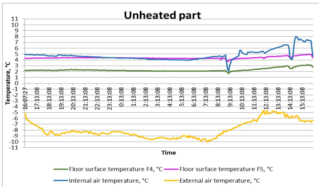
Figure 3 The time course of measured floor surface temperatures in unheated part of the repair indoor object and internal and external environment temperatures
