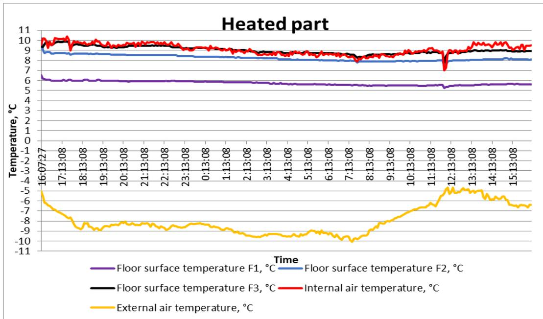
Figure 2 The time course of measured floor surface temperatures in heated part of the repair indoor object and internal and external environment temperatures
