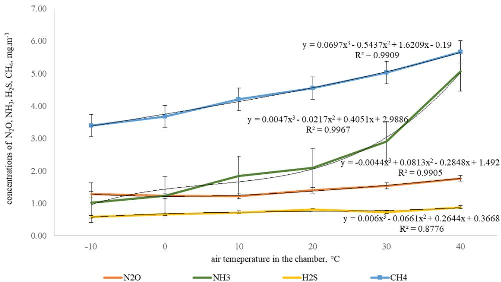
Figure 3 The course of gas concentrations in climatic chamber in raising of the air the temperature - measurement of the wet RMS
