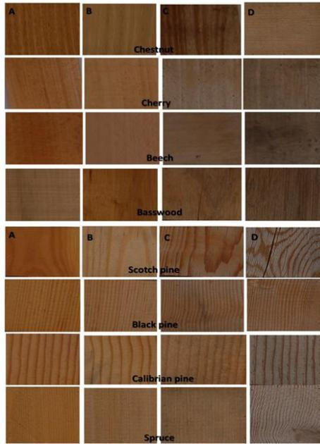
Fig. 2: Surface natural appearance of wood species at various conditions: A- Control, B- one month, C- six months, D- 12 months of natural weathering durations at outside.
