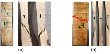
Fig. 2: Failure pattern under compression and tension for Eucalyptus camaldulensis (Safeda) from city of (a) Sheikupura, (b) Khushab.
