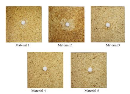
Fig. 5: Damage views of the impacted bio-composites.
