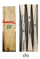
Fig. 4: Failure pattern under compression and tension for Albizia lebbeck (Shreen) from city of (a) Sari Alamgir, (b) Gujranwala.
