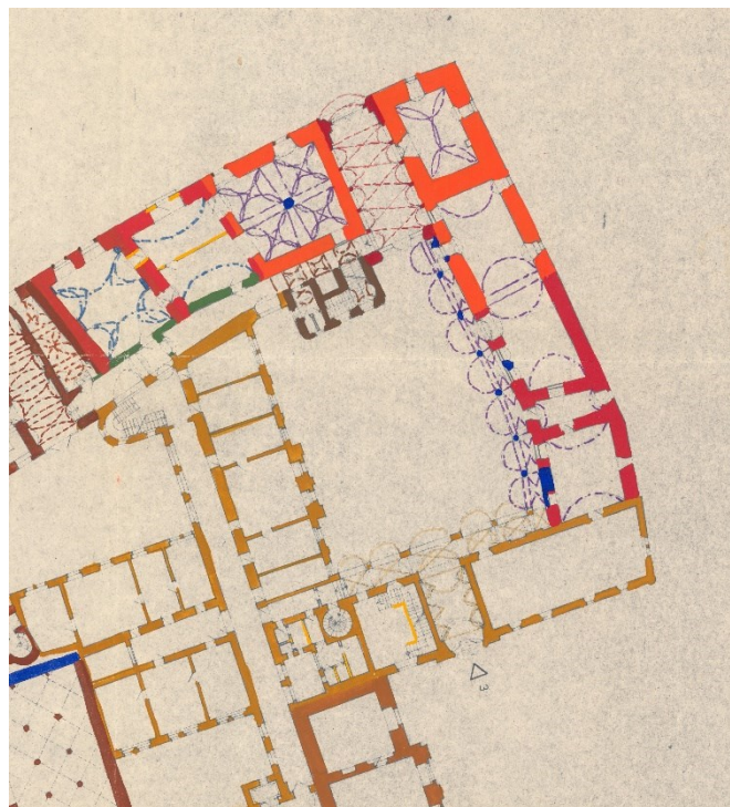
Fig. 1. Floor plan of the Old Town Hall with development stages marked. Author: Peter Kresánek. (Source: Municipal Institute for the Protection of Monuments in Bratislava, Slovakia, Department of Documentation, Inv. Number 1719, Fig. 2.)
