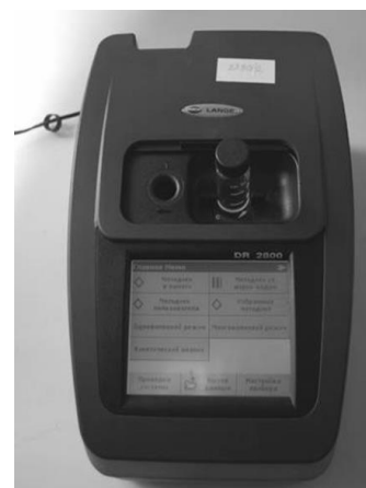
Figure 9 Spectrophotometer SDR 2800 by Hach
