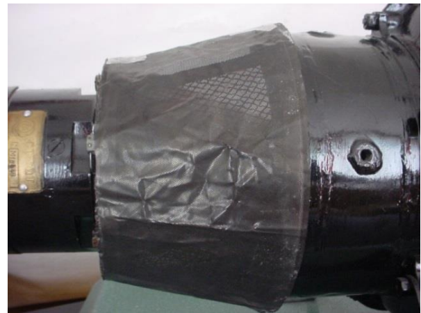
Figure 12 Perforated plates attached to the original inlet device of MPM-20
