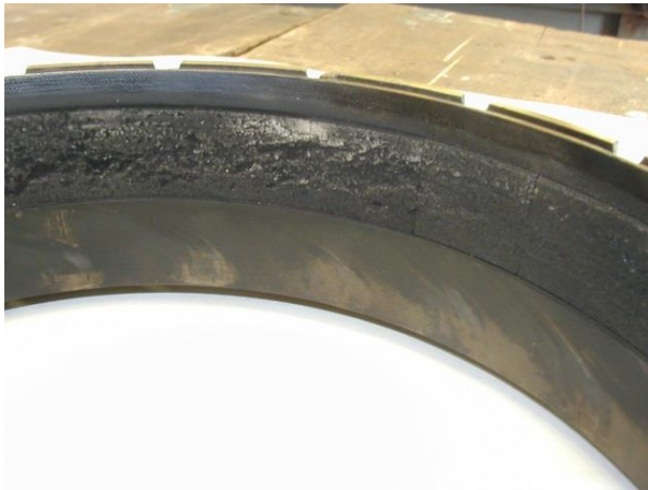
Figure 14 Tanned seal in gas turbine housing
