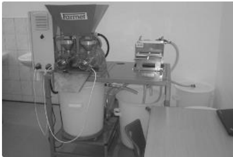
Figure 11 Laboratory of liquid and solid fuels with pressing, filtering and mixing equipment by Farnet Company
