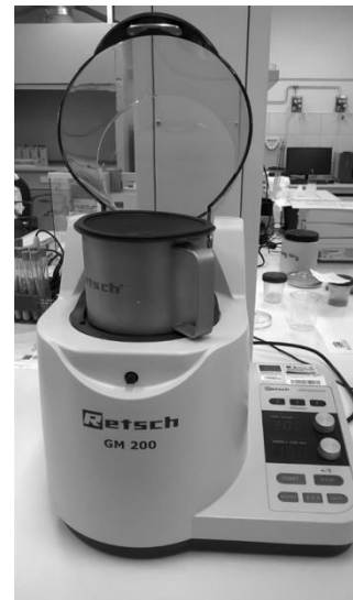
Figure 5 Grindomix GM 200 homogenizer by RETSCH
