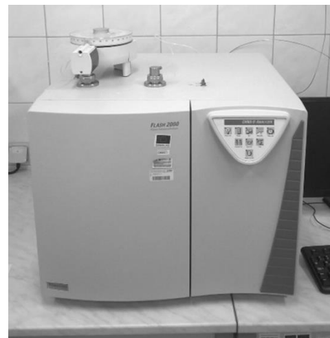
Figure 6 CHNS(O) analyzer Flash 2000 by Thermo Scientific
