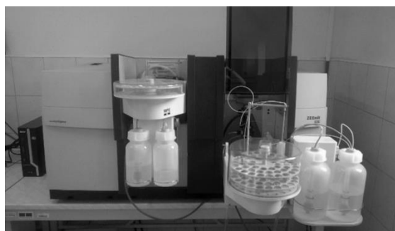
Figure 8 Atomic absorption spectrophotometer by Analytic Jena AG
