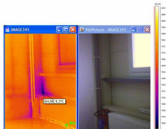
Figure 4 Course of surface temperatures in the corner of peripheral case (outdoor temperature of air +2°C)[5]
