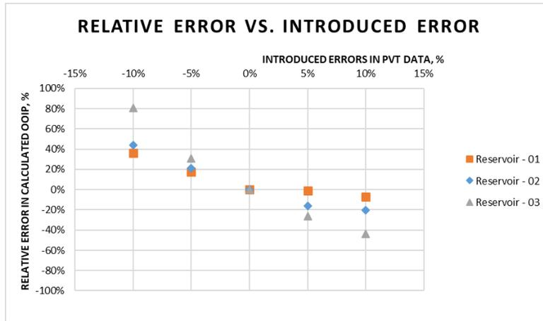
Figure 7. Relative errors in calculated OOIP vs. introduced errors in PVT data
