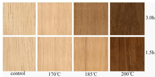
Fig. 1: The color variation of the surface between untreated and thermal modified rubberwood.
