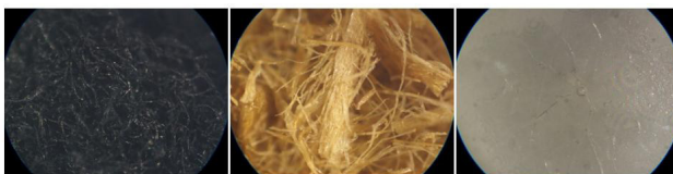
Fig. 4: Pure fibres: a) original, b) after STA, c) after furnace.
