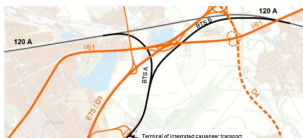
Fig 4. Proposal for the connection of the terminal of integrated passenger transport of the M. R. Štefánik Airport to the ŽSR 120A track section (Source: Remeň, 2019)
