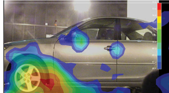
Fig. 2. Acoustic map of the vehicle with the engine running in the wind tunnel (Burdzik, 2012)
