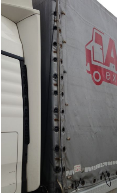
Fig. 6. Freight vehicle with totally unfolded tarpaulin on side part of the body
