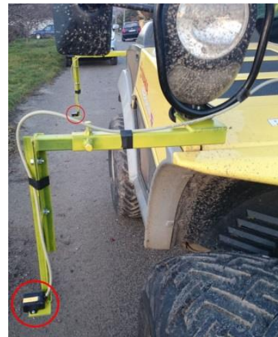
Figure 2. Dislocations of acceleration sensors on machine
