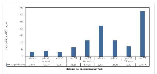
Figure 2 Average CH<sub>4</sub> production in V1, V2 and V3 pile in the first, fourth and seventh week after piles creation
