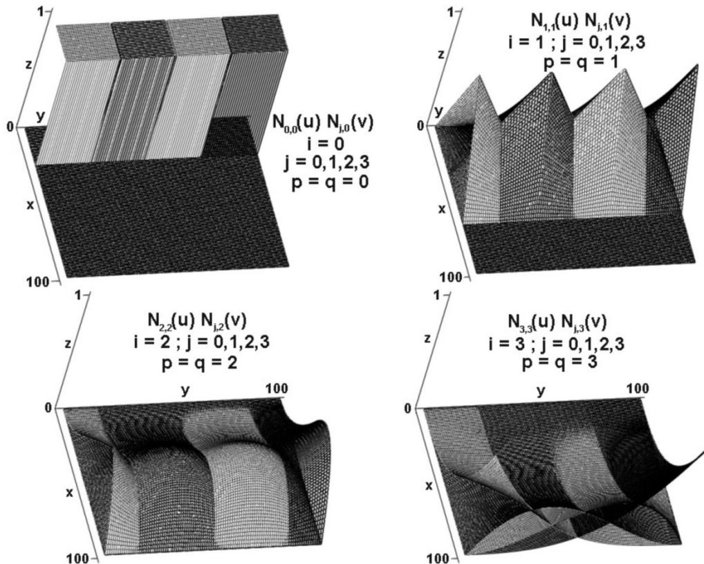
Fig. 1 Basis functions of the B-spline surface.
