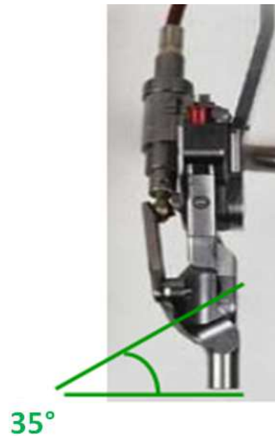
Figure 4 Axis joint with 35 ° inclination
