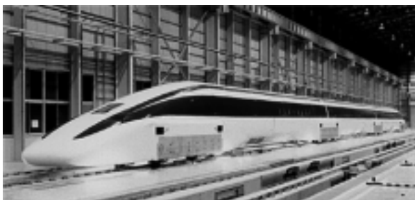
Fig. 7. Vehicle MLX01, being operated unmanned for testing up to 550 km/h [8]
