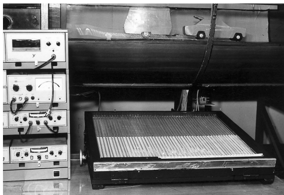
Obr. 3. Model auta s karavanom vo veternom tuneli Fig. 3. Model of automobile with caravan in a wind tunnel of DSM CEF UZ
