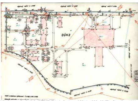
Fig. 6: A land survey sketch of the OÚNZ (District Institute of National Health) Topolčany from 1981 to a scale of 1:1000 after the construction of the new hospital complex (Cadastre Section of the Topolčany District Office) (KoOÚ Topolčany, Land surveyor sketch of the OÚNZ Topolčany to a scale of 1:1000, 1981.)
