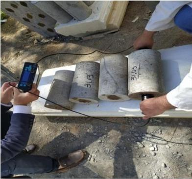
Figure 2: Ultrasound pulse velocity measurement (direct transmission performed on field-cured specimens)
