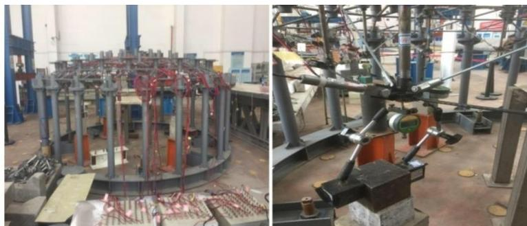
Figure 3: Construction and deflection dial indicator layout
