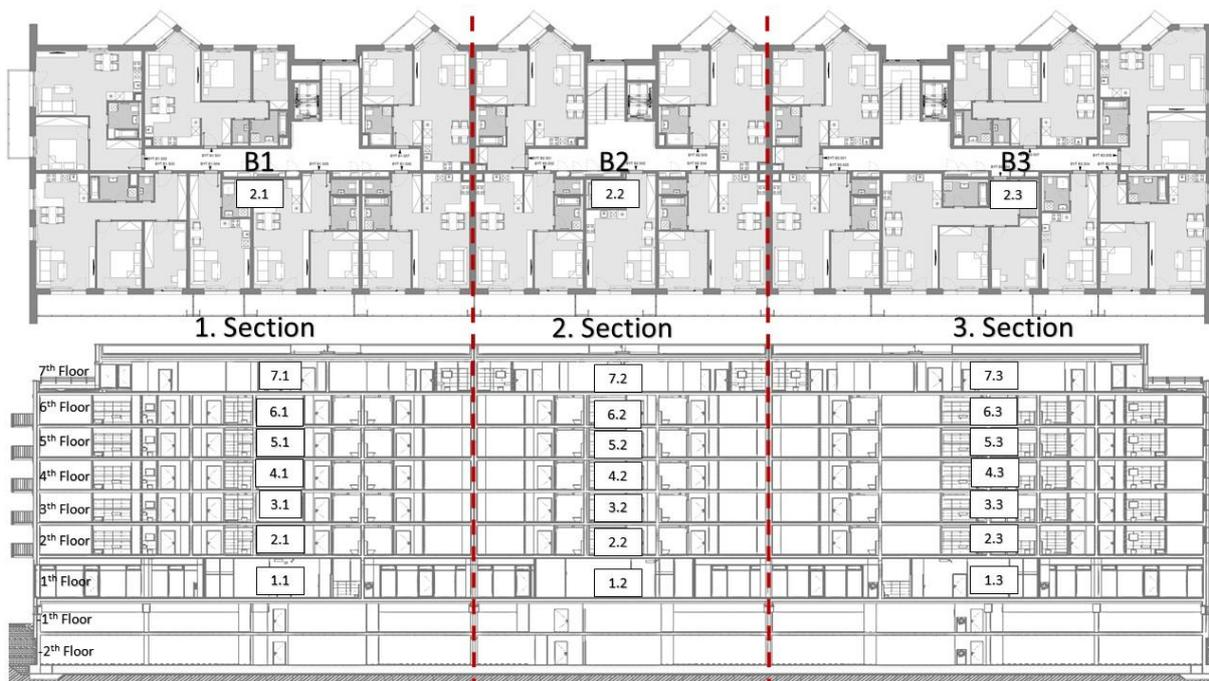
Figure 1: Case study residential complex Popradská: apartment building "B", divided into three sections with marked work zones: (a) 2.th Floor plan, (b) section C-C [15]
