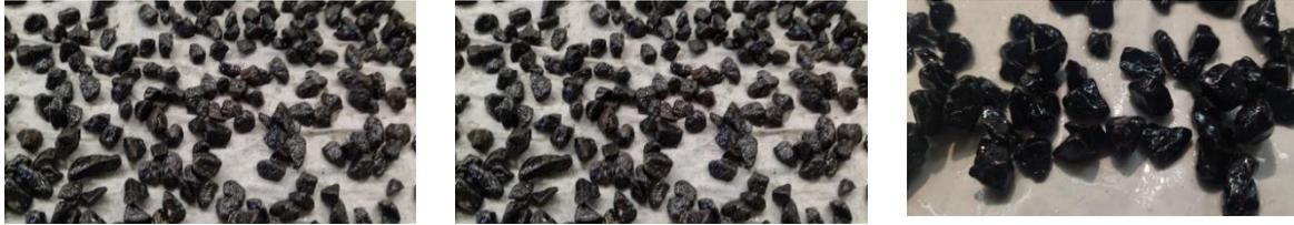
Figure 4: Affinity tests between aggregate and net bitumen type CA 50/70 (left), net bitumen type CA 50/70 modified with commercially available LDPE (centre) and net bitumen type CA 50/70 modified with LDPEre (right)
