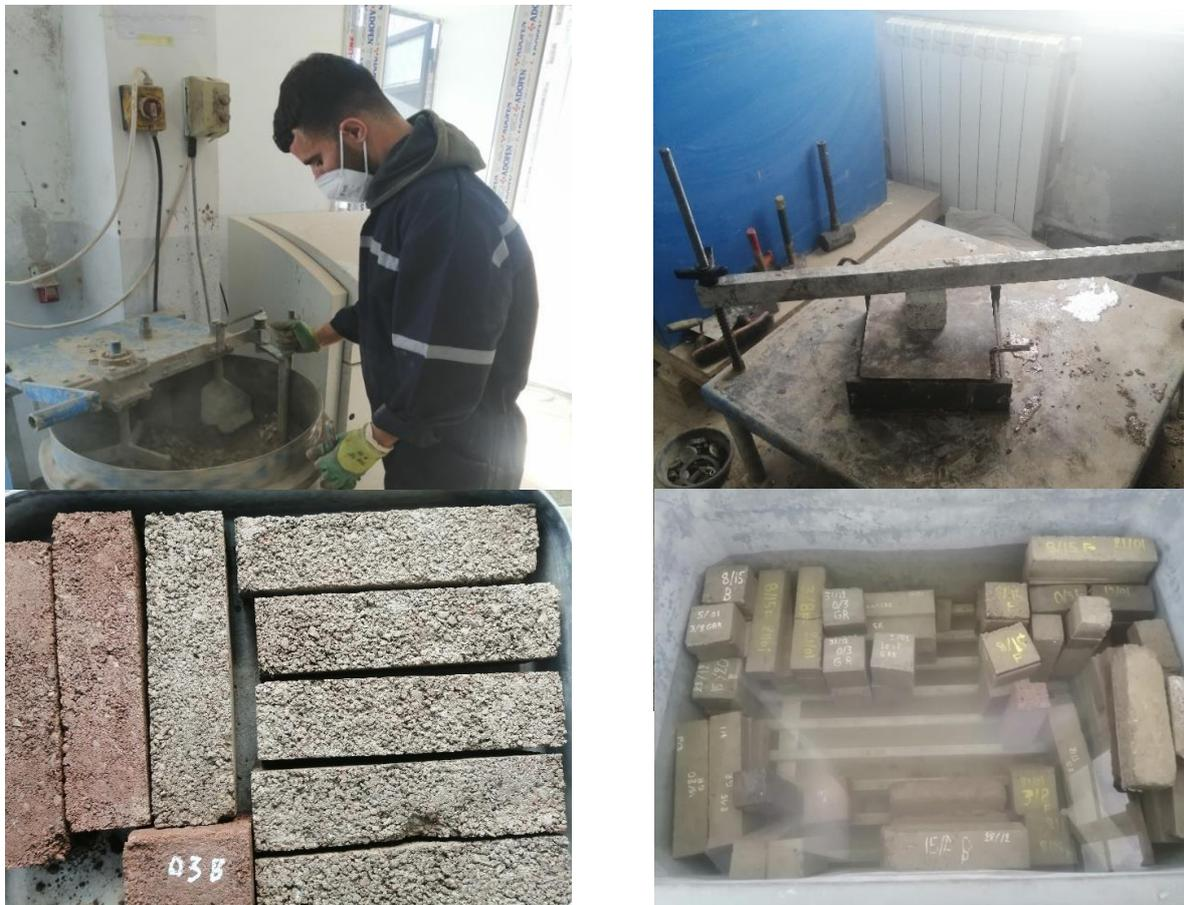
Figure 3: Method for preparing the mixtures of CTB
