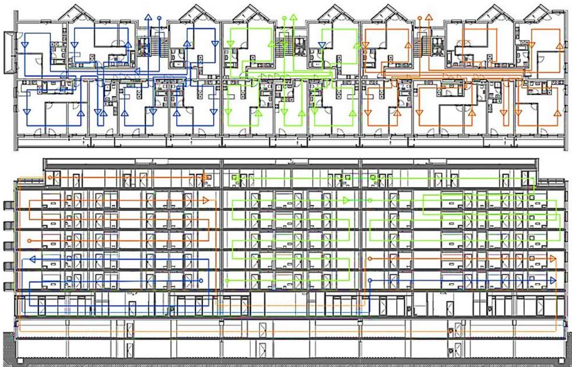
Figure 3: The results of mapping the direction of the plastering work of individual work teams on a typical plan of the 3<sup>rd</sup> floor and in section ( — - team № 1, — - team № 2, — - team № 3)
