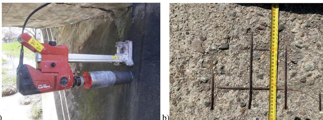
Figure 3: a) Sampling from the middle pillar, b) reinforcement at the upper surface above the pillar
