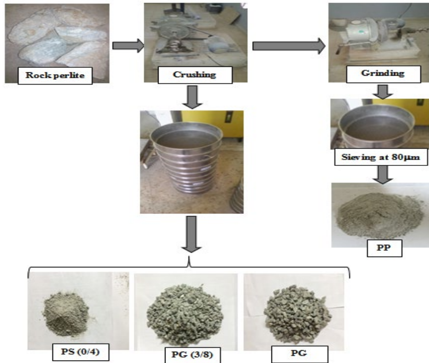
Figure 2: Stages of rock perlite recycling
