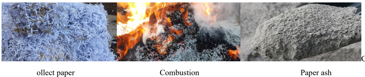
Figure 2: The stages of preparation of industrial waste
