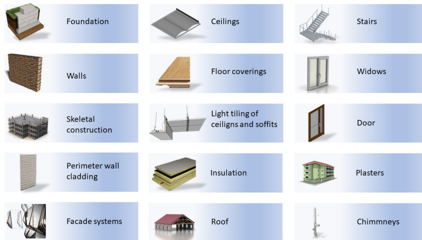
Figure 2: Division of the construction into functional parts
