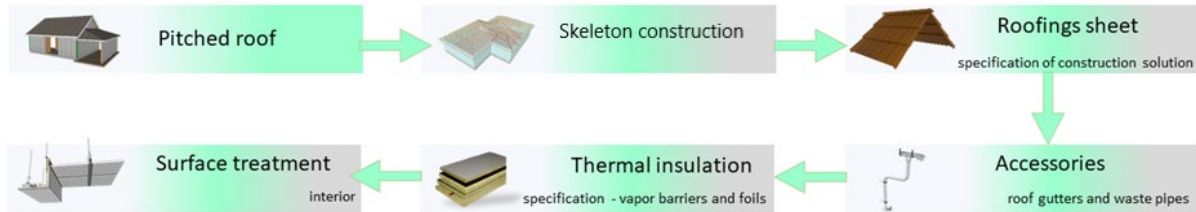
Figure 3: Flowchart – creating a pitched roof detail
