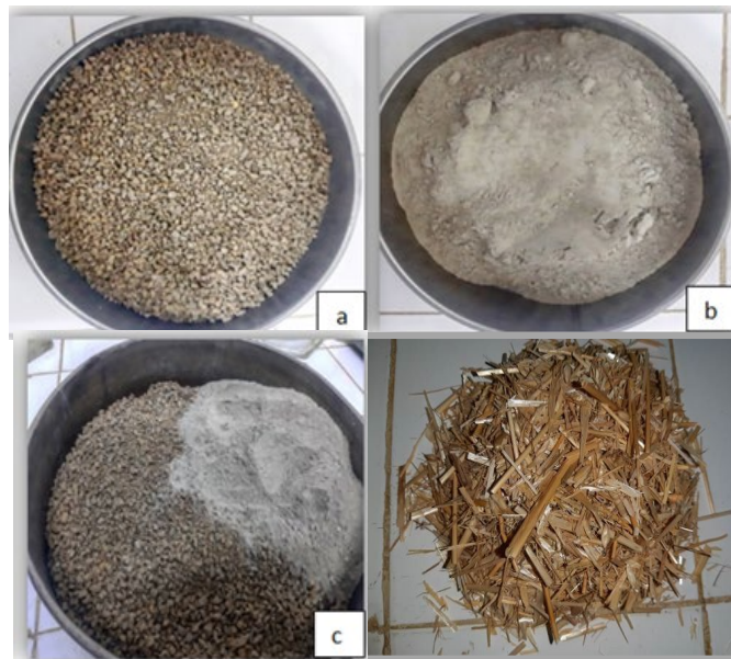
Figure 3: a) Natural soil; b) Bentonite; c) Reconstituted soil (60% natural soil +40% bentonite); d) Wheat straw
