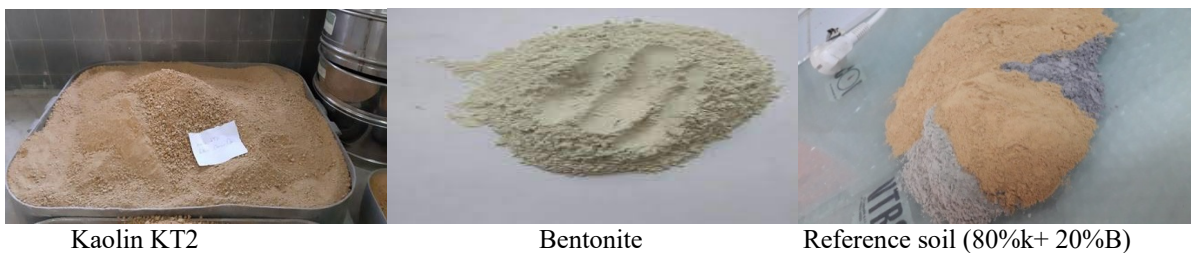
Figure 1: The reference soil components
