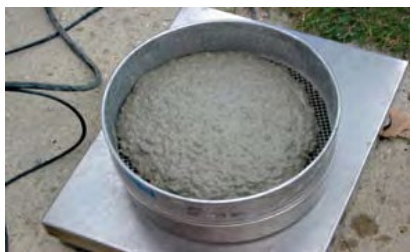
Sieve segregation test
