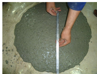
Slump flow test
