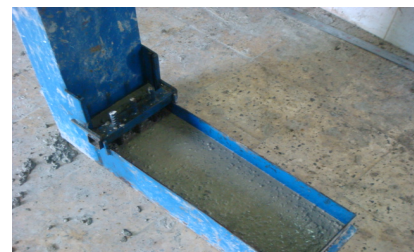
L Box blocking test
