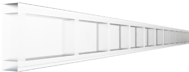
Figure 2: Transparent wood Vierendeel box beam rendering [8]
