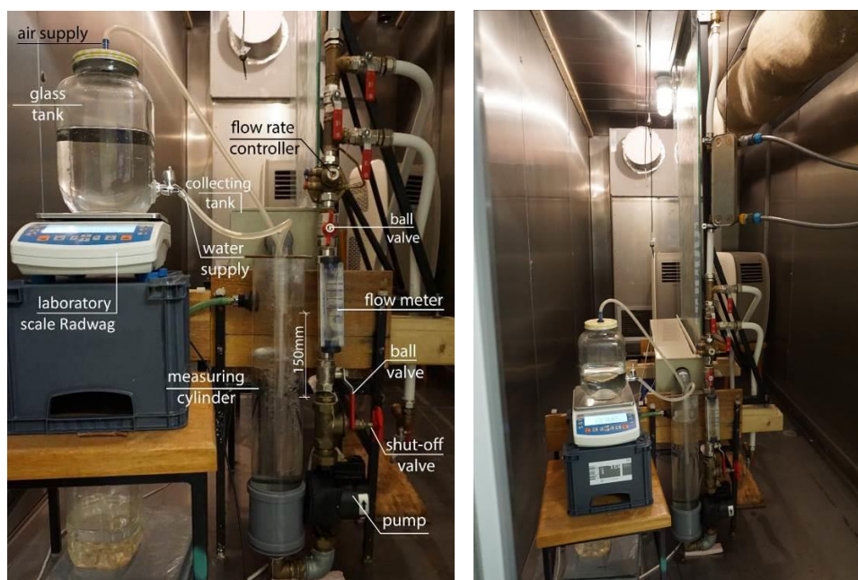
Fig. 4: Measuring system of evaporation performance
