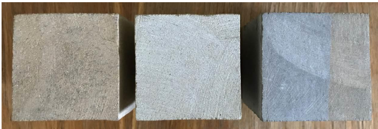
Figure 11: Samples of sandstones top view : from the left: Kežmarok, Stará Ľubovňa - Kremná, Spišské Tomášovce
