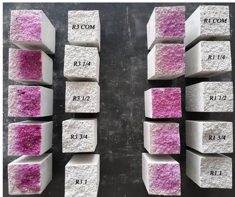
Figure. 2: Samples of formula R3 and R1 after the application of phenolphthalein on the fracture surface.
