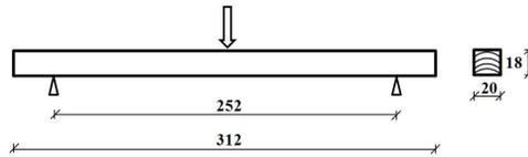
Fig. 3: Schematic diagram of the bending test.
