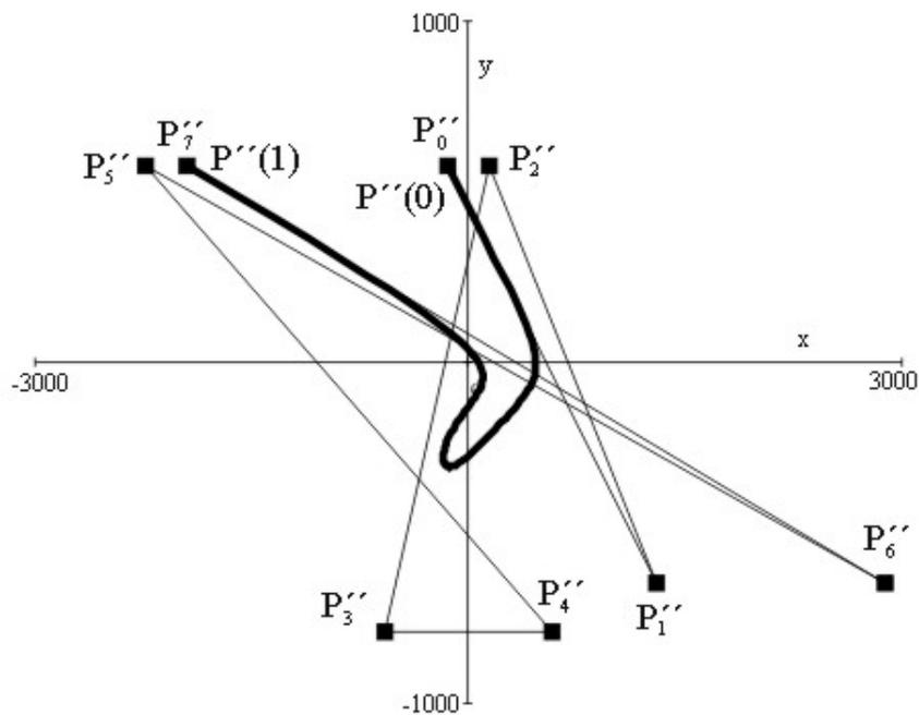
Fig. 3 The second derivation of the Bézier curve with its control points
