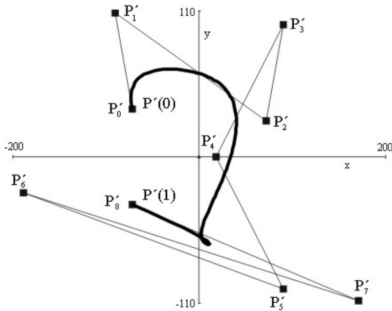
Fig. 2 The first derivation of the Bézier curve with its control points
