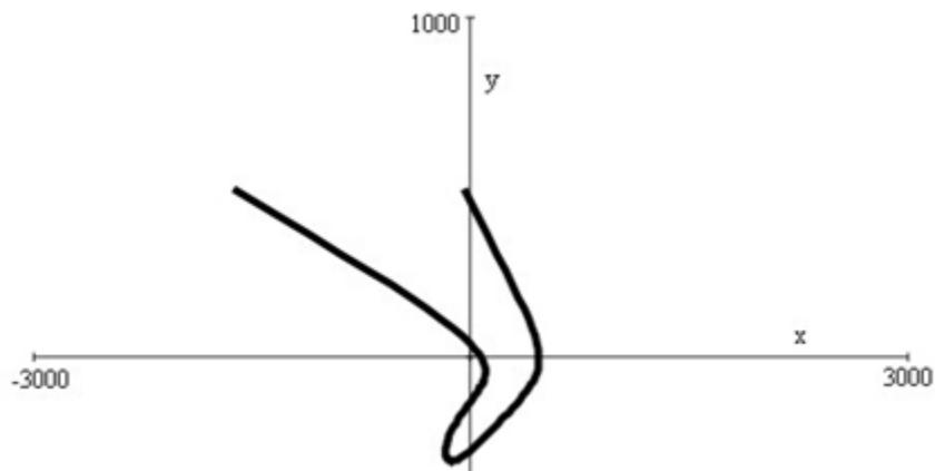
Fig. 5 The second derivation of the Bézier curve with its control points.
