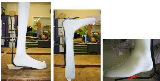
Figure 6 Positioning of the carbon spring on the plaster positive
