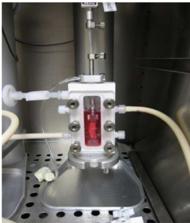
Figure 1 A commercially available bioreactor is depicted in this image (DynaGen bioreactor system, Tissue Growth Technologies, Minnetonka, MN, USA) [14].
