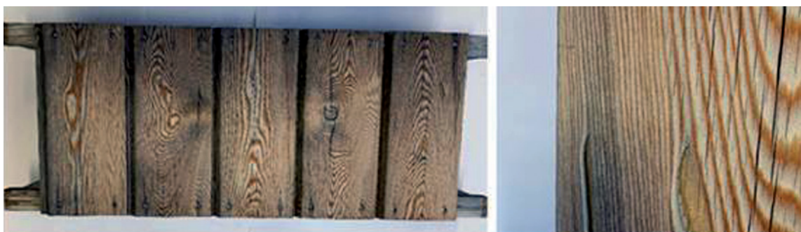
Fig. 9. The formation of cracks – visual appearance of Siberian larch after 12 months of exposure to south side, construction type A.
