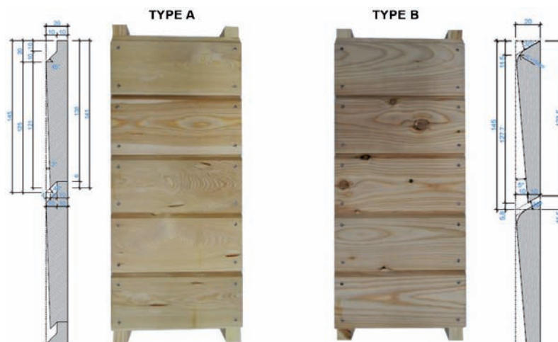
Fig. 1. Design of facade profiles – type A (left – Siberian larch) and B (right – European larch). Type A is characterized with cladding top cut in 45°, while type B was designed with inclination 30° and rounded top with radius r = 15 mm.
