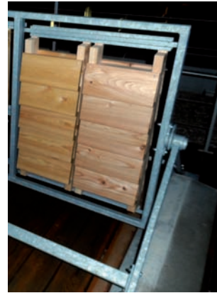
Fig. 2. The placement of facade models in the testing stands in exterior in 90°.
