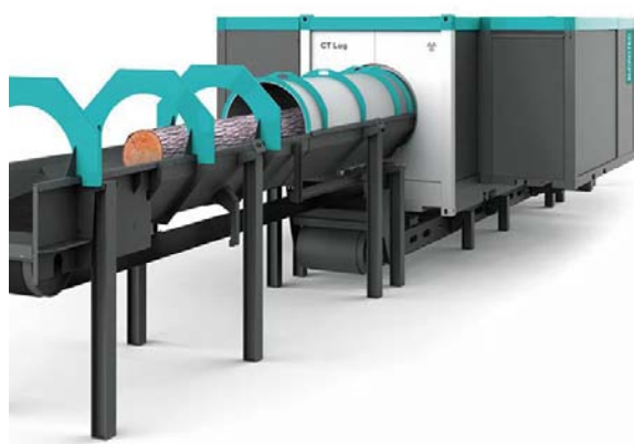
Fig. 5. CT Log scanner. © Microtec (Microtec 2019).
