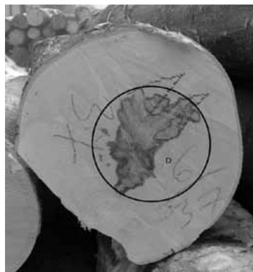
Fig. 1. Evaluation of false heartwood on beech according to STN EN 1309–3.
