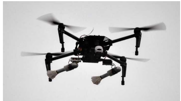
Fig. 1 Conventopnal UAV with improvised ammunition
