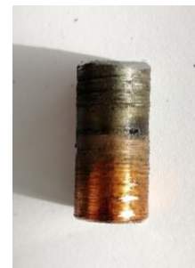
Figure 3 Heterogenous friction weld steel 23B2 - copper, modified specimen [1]
