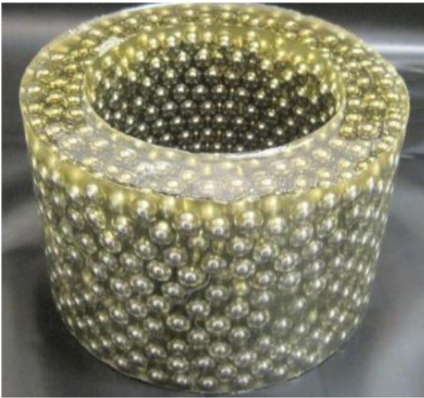
Fig. 5 Matrix with fully formed shrapnels
