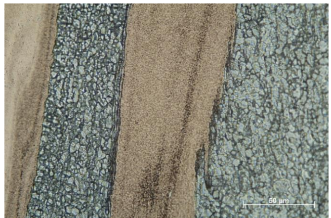
Figure 6 Microstructure detail of heterogeneous friction weld steel 23B2 – copper [1]
