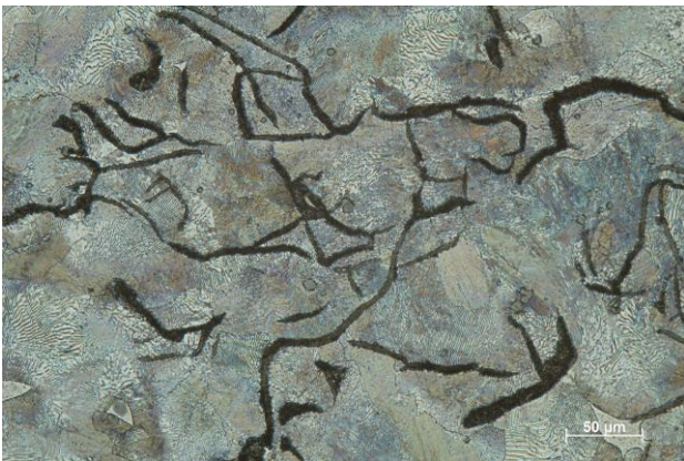
Fig. 8 Structure of grey cast iron for comparing with the structure of M390 a M398
