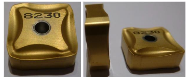
Fig. 2 Geometry of tested cutting inserts used in the face milling process
