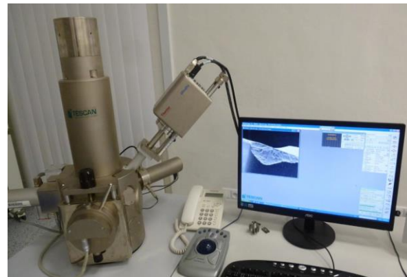
Fig. 5 View of a scanning electron microscope type Tescan VEGA 5135 with X-Ray microanalyzer Noran Six / 300, which was used in the experimental process to monitor the final wear of tested cutting plates type SNHF1204ENSR-M during face milling process of Armox 500 steel
