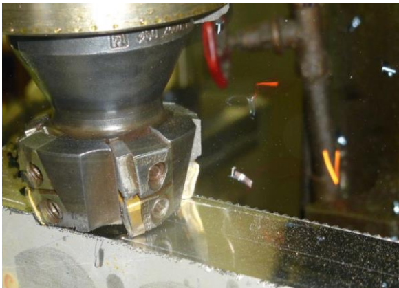
Fig. 4 View of the face milling process at a cutting speed v_c = 111 \text{ m} \cdot \text{min}^{-1} (machine spindle speed n = 710 \text{ min}^{-1} ), depth of cut a_p = 2 \text{ mm} , and feed rate per tooth f_z = 0.056 \text{ mm}
