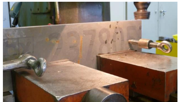
Fig. 3 A look at the method of clamping 2 pieces of ARMOX 500 sheets, using two machine vices on a FA 3V machine tool
